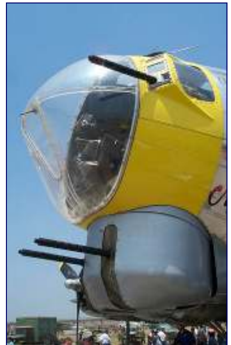
The chin turret of the B-17G and the left cheek gun. The powered chin turret, operated by the bombardier, greatly improved the B-17's forward defenses.
